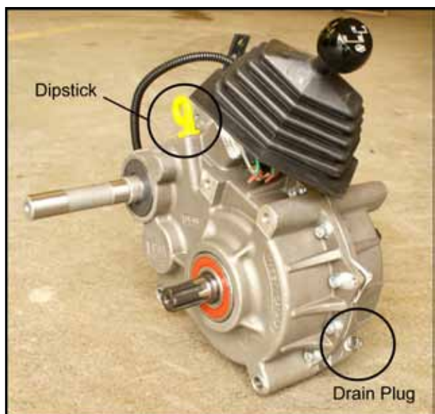
Figure 6-4a. 34-100 Transmission showing dipstick and drain plug locations
