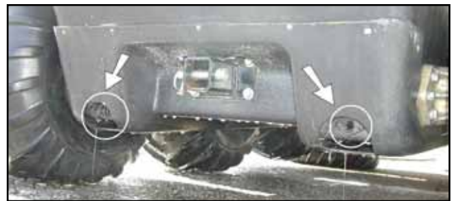
Figure 5-1. Location of rear drain plugs.
