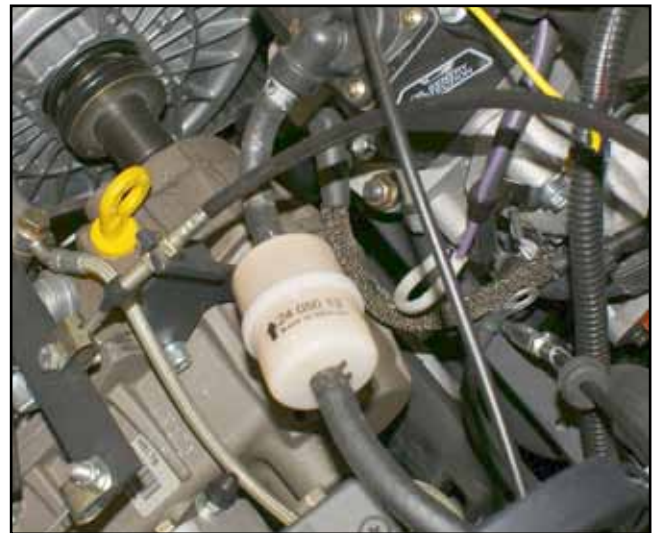
Figure 6-6a. Avenger 700 fuel filter location.
